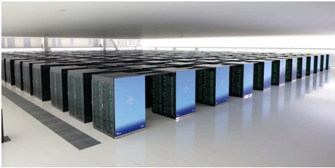
Modern devices powered by ARM architecture (RIKEN Fugaku (2020) World's most powerful Supercomputer in 2020)
